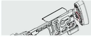
**Step 2:** Slide the buttpad up or down in 1/4" increments, or cant it 15 degrees to either side. There are protrusions on the aluminum LOP bar that fit into pockets on the polymer buttpad housing, assuring positive lock up. Retighten Thumbscrew when desired position is achieved.
