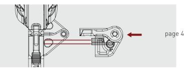
Step 6: Apply a small amount of blue Loctite to the M6x25mm button head screw and M6x18mm flat head screw and attach top hinge to the chassis.
