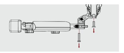
**Step 2:** Remove the top hinge, ensuring both pins remain inside the hinge. The smaller-diameter pin secures the secondary release button in place and should not be removed.
