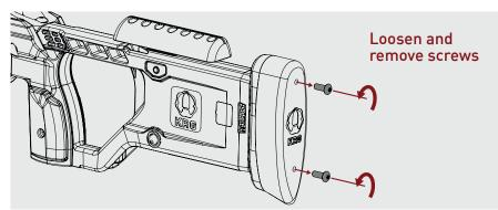
**Step 2:** Replace these screws with included longer screws, corresponding to the desired number of spacers.
